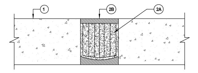
Wall Assembly – Min 5 in. (127 mm) thick reinforced lightweight or normal weight (100 – 150 pcf or 1600-2400 kg/m³) structural concrete. Wall may also be constructed of any UL Classified Concrete Blocks\*.
